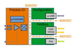
In the RAIL version, the CAN bus and the power supply are routed in the same cable. Here, the ground potential of the power supply is identical to that of the CAN bus. The isolation to the process IO is designed for 1.7 kV DC.
