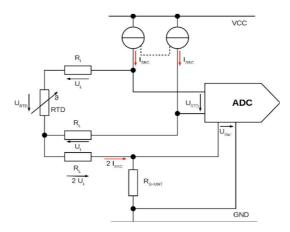
The 16-bit AD converter used directly measures the ratio between the voltage at the sensor and the supply current, i.e. the actual resistance value. A switchable gain factor allows optimized adaptation to Pt100 or Pt1000 sensors.
